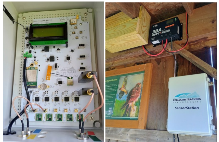
Some of the inner workings of the Motus bird tracking station: the battery controller (left) and the Sensor Station (right). The equipment will read the radio tags of birds flying overhead and contribute it to the world-wide Motus database. Visit it at www.motus.org . Photos: John Loz.
